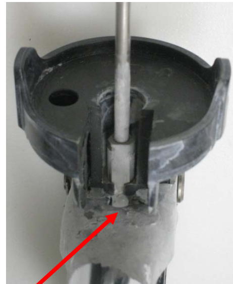
Leaking of material due to a failure of seal In Atomizing Head
