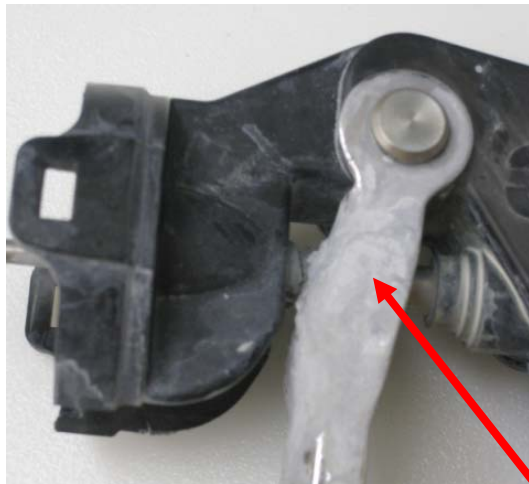
Leaking of material due to a failure of seal In Atomizing Head
